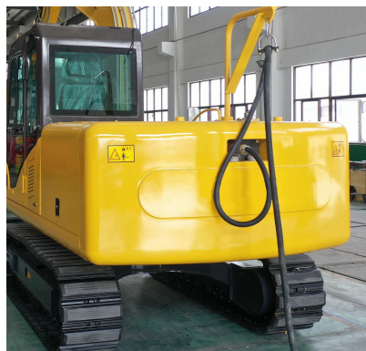
Cable Power Supply
